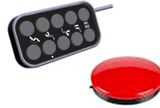
Figure 20: Direct access switches
