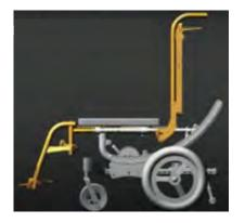
In this case, completing the CG-CR adjustment will move the seating system forward relative to the caster wheels, impacting the front stability.
